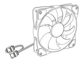
To RGB header (only one needs to be connected)
